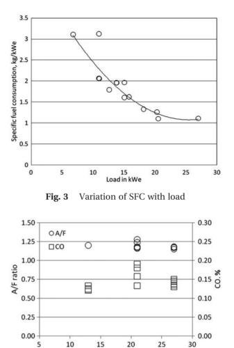
**Fig. 4** Variation of air-to-fuel ratio in the mixture and CO in the exhaust with load
