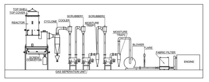
Fig. 1 Schematic of the open-top down-draft gasification system
