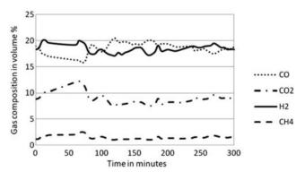
Fig. 2 Gas composition with time
